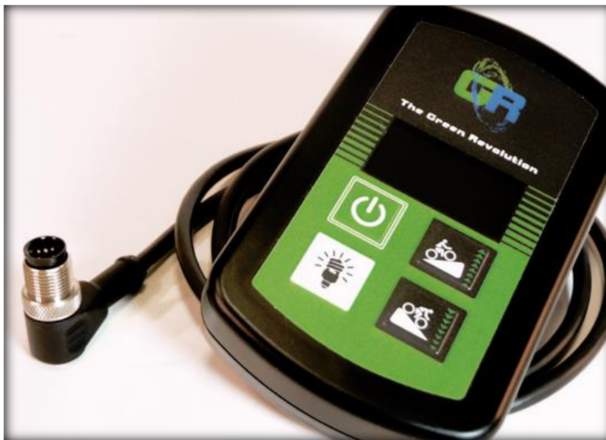
Figure D3.1: Handheld device for increasing resistance and monitoring energy output of biker.
